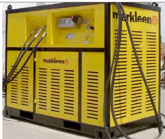
Fig. 9 Hydraulic power pack Markleen DHPP 60
